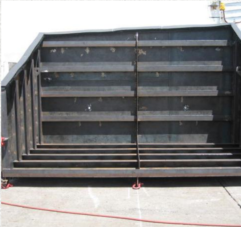
Surface Piercing Cofferdam Interior
