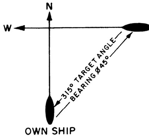
Figure 10.—Target angle.
