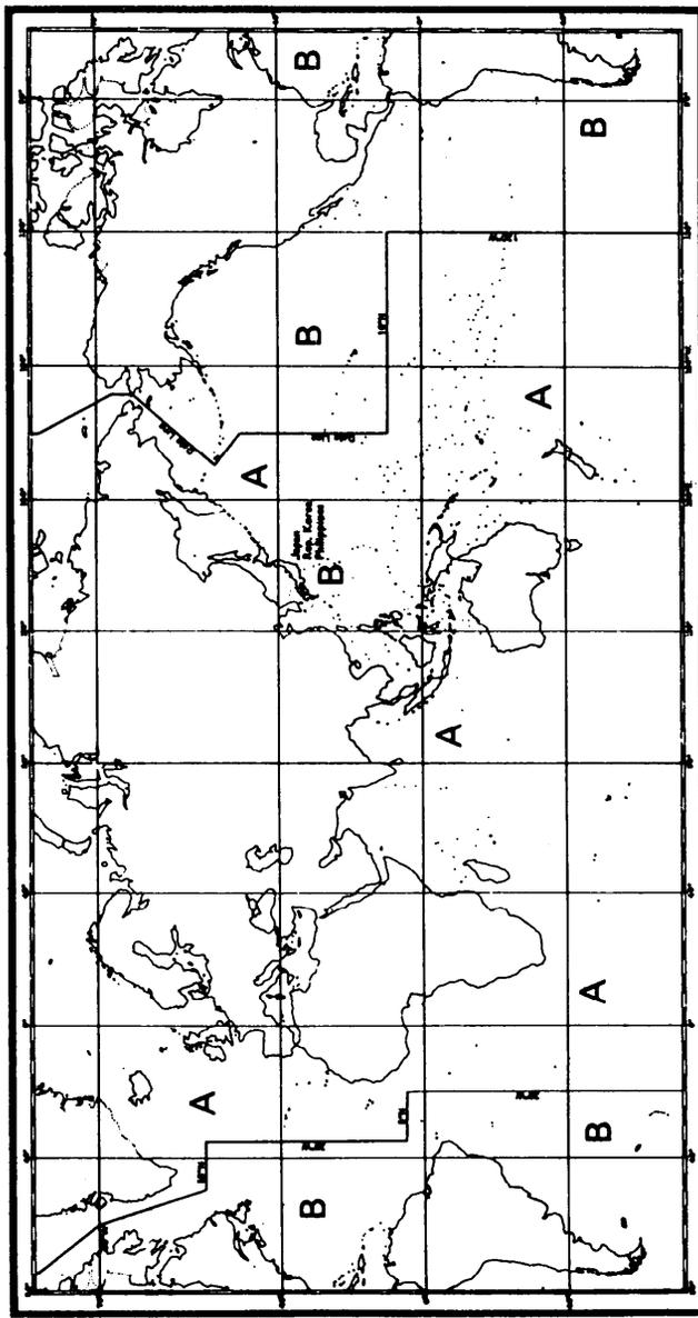
Figure 22.—IALA Maritime Buoyage System; buoyage regions A and B.
