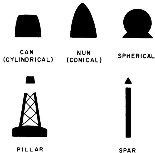
Figure 23.—Basic buoy shapes.
