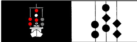
VESSEL ENGAGED IN DREDGING OR UNDERWAY OPERATIONS WHEN RESTRICTED IN ITS ABILITY TO MANEUVER; SHOWING CLEAR AND OBSTRUCTED SIDE.
